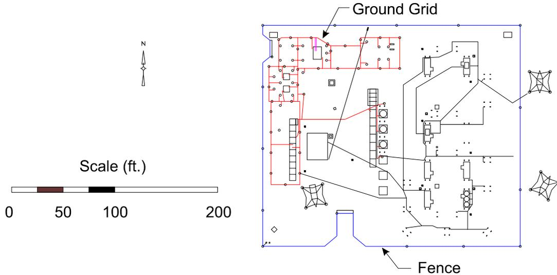
Figure 1 General arrangement of equipment and ground grid of Station “OK”
