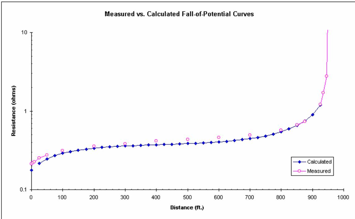
Figure 12 Fall-of-Potential curve comparison.
