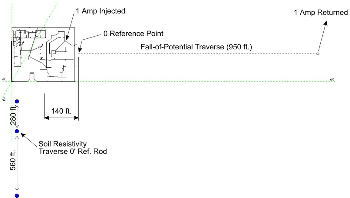
Figure 2 Location of fall-of-potential and soil resistivity measurements
